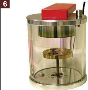
6. Evaporate a thin layer of gold using a sputter coater. 30 ma for 30 seconds at a working distance of approximately 5 cm is sufficient.
