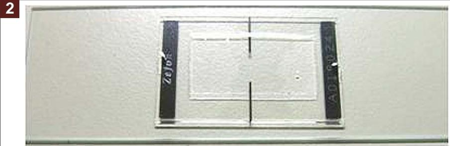
2. Remove the CSI coverslip from the cassette and mount on a microscope slide with the particle collection side facing up. Place a section of screen mesh or a TEM finder grid directly over one side of the sample trace if direct comparison analysis is desired. Apply stain and a coverslip and analyze the slide according to normal optical microscopy procedures.
