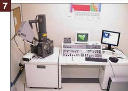
7. Place the sample into the SEM and relocate and analyze the particles of interest.
