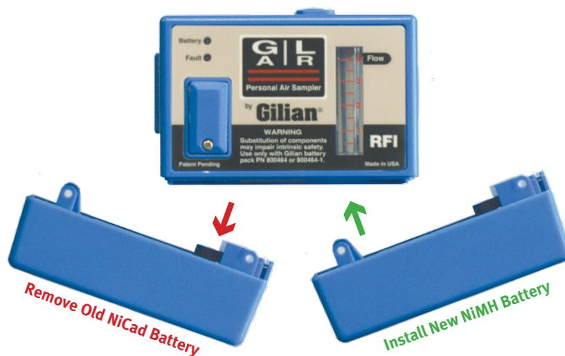
**Upgrading your GilAir-3 or GilAir-5 to the new NiMH batteries requires no pump changes; simply exchange the battery pack.**
