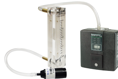
INCORRECT setup with sampling media at the end of the sample train
