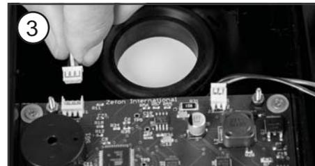
Unplug the old battery from the circuit board. Remove it from the top of the case.
