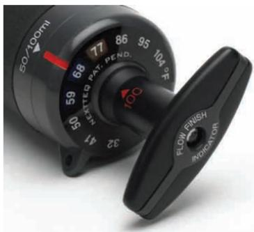
The Thermal Ring, which is affixed to all new Gastec GV-100 pumps, is perfectly calibrated to work with the Gastec Gas Sampling Pump and Detector Tube Systems. Please see other side for instructions on affixing the Thermal Ring and warning label to a GV-100 pump in the field.
