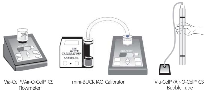
The Via-Cell flowmeter used with the Zefon Bio-Pump® has the in-line resistance of a sampler built into the calibration scale. When using the mini-BUCK or Via-Cell/Air-O-Cell CSI bubble tube, actual samplers are used in-line during calibration. For complete calibration instructions, please refer to the instructions included with your pump or calibration device.
