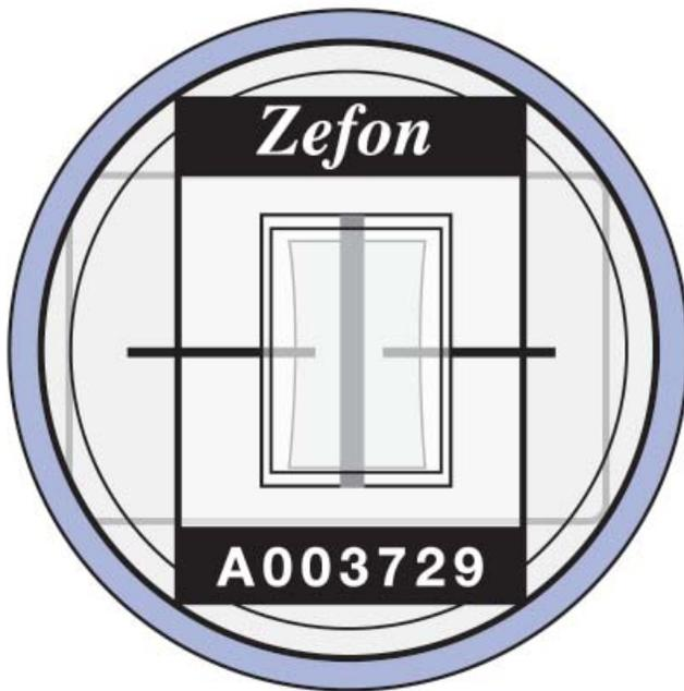
4. Put 2cc sterile water into the trough in the bottom half of the cassette. After cleaning the tweezers tip with alcohol, place the slide upside down (media side down) on top of the water. If any large bubbles are trapped under the slide, gently lift one side of the slide and slowly lower to remove bubbles. **NOTE: Be sure the alcohol has completely dried before handling the slide.**
