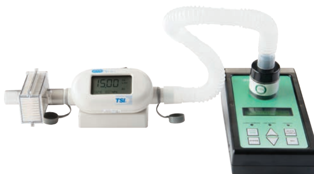
Bio-Pump connected to a TSI Flow Calibrator
