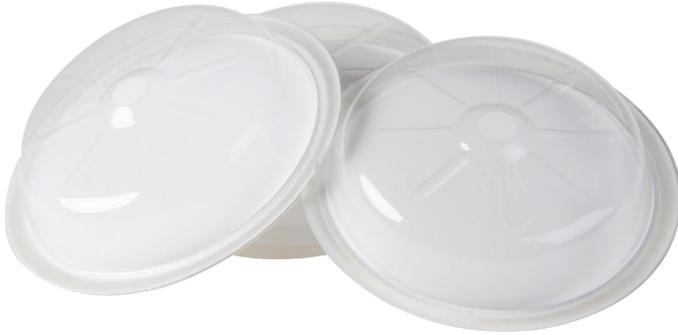
The Solu-Sert™ filter capsule is a self-contained filter “cassette capsule” that captures all particles that enter a filter cassette. It consists of an MCE filter membrane sealed to a cellulose shell to create the capsule. This capsule is then inserted into a Zefon 2-Piece filter cassette with a support pad as a complete unit. After sampling, the entire capsule is removed, digested, and analysis performed.
