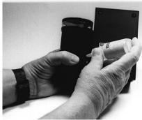
C. Wet flow cell by connecting a pump flowing at 1000 to 2000 cc/min. Initiate soap film up center tube by rapidly pressing button down and releasing. Repeat this procedure until bubble doesn't break. The tube is now wet and tests at any range may be conducted. One minute warm up time is all that is required of the DigiCal.
