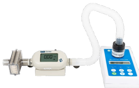
TSI 4046 Primary Calibrator connected to pump.
